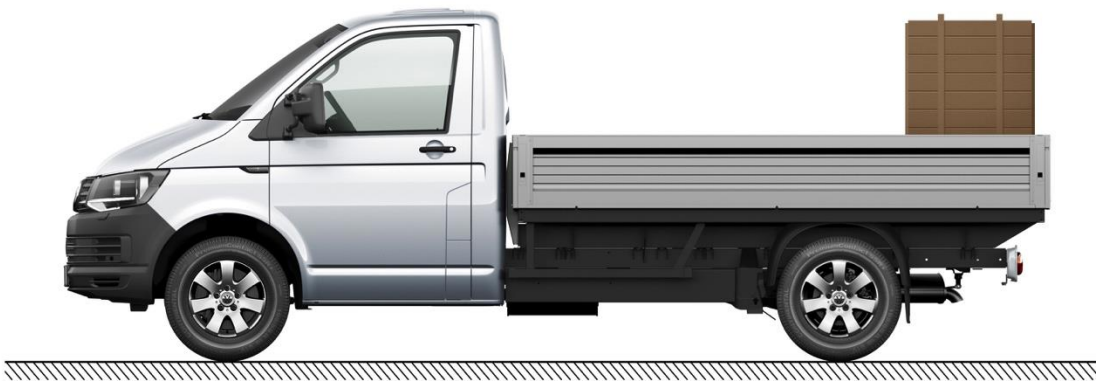
Fig. 2: One-sided weight distribution (side view)
