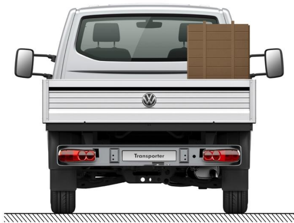
Fig. 1: One-sided weight distribution (rear view)
