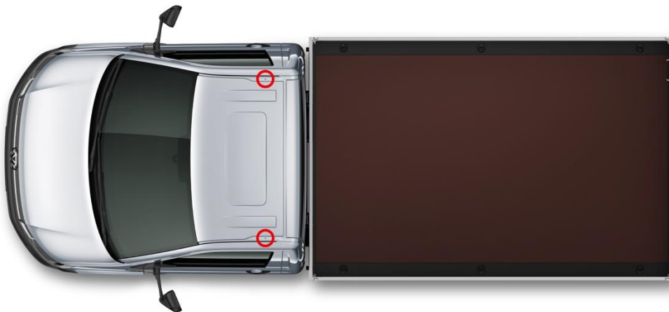
Fig. 3: Standard roof fastening points for single cabin
