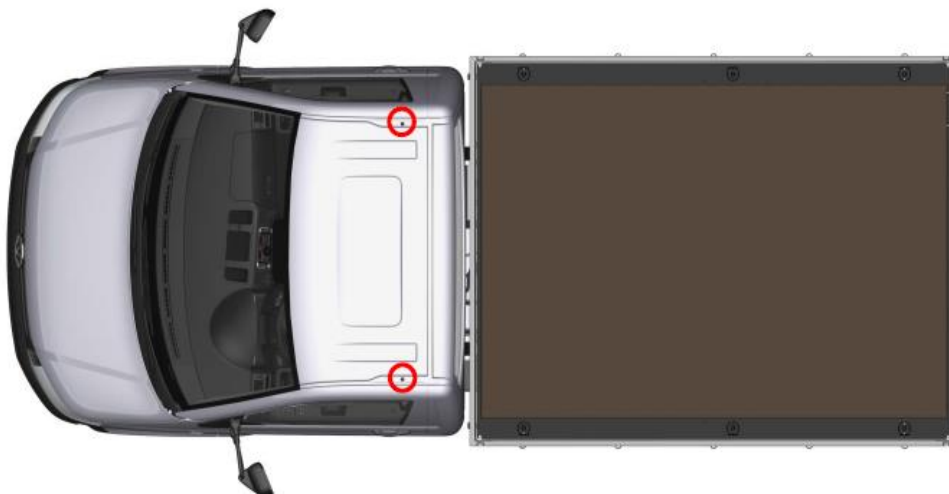
Fig. 3: Standard roof mounting points in platform van
