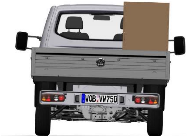
Fig. 1: One-sided weight distribution (rear view)
