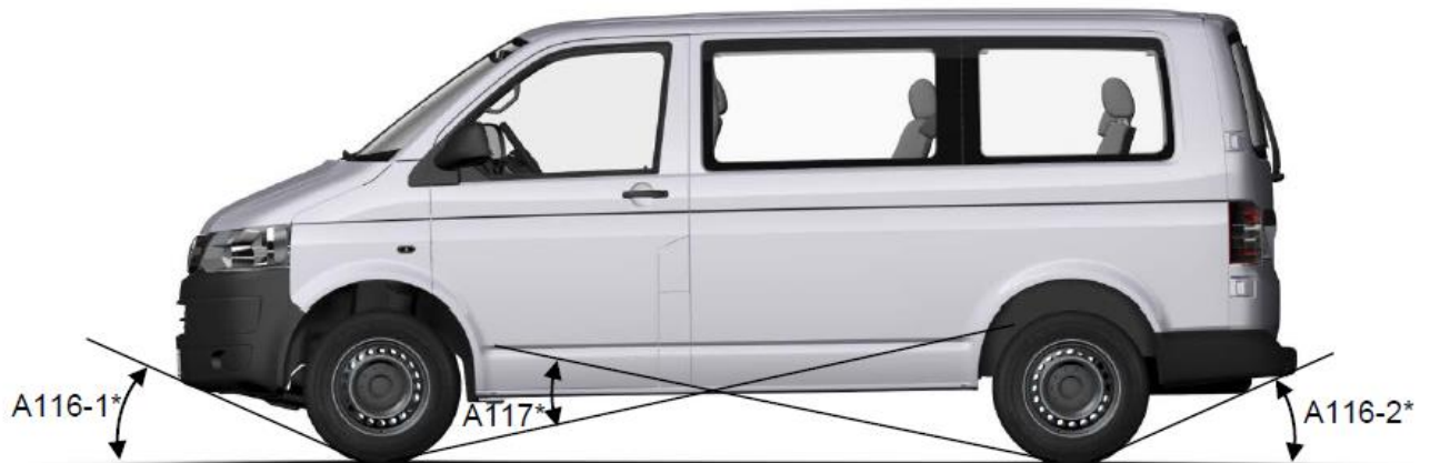
Fig. 1 Overhang and ramp angles, Transporter panel van/window van
