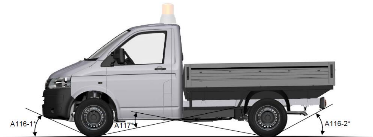
Fig. 2 Overhang and ramp angles, Transporter platform van/chassis
