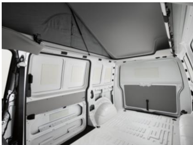
Fig. 1 and 2: Pop-up roof with large roof cut-out
