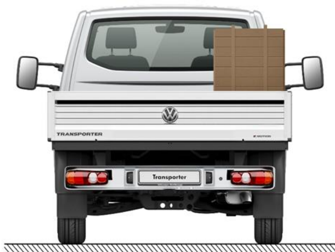
Fig. 1: One-sided weight distribution (rear view)
