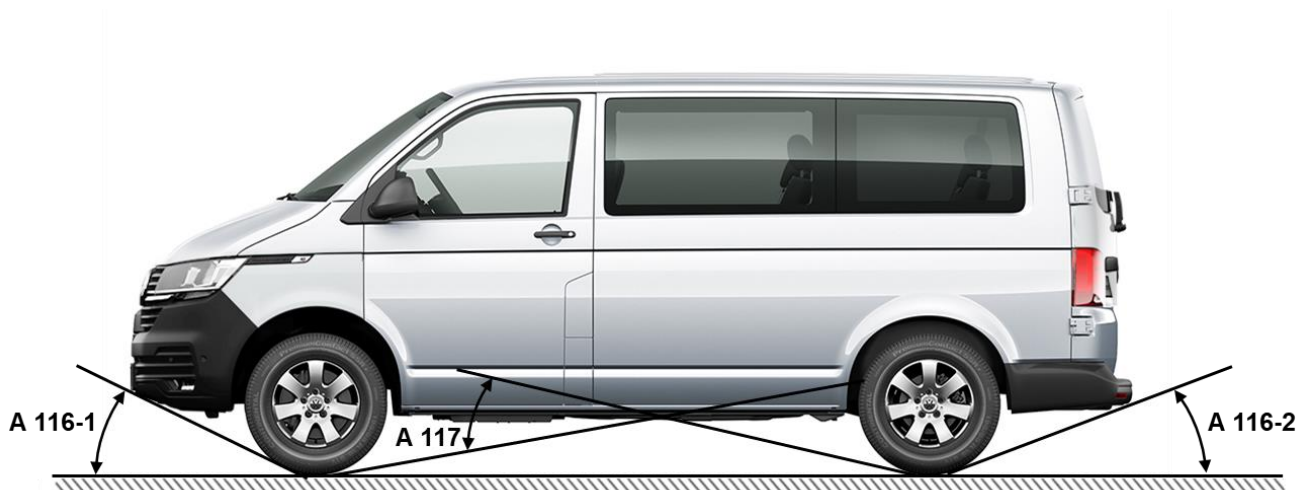
Fig. 1 Example ramp angle and breakover angle of Transporter panel van / window van with short/long wheelbase (acc. to DIN70020, T1)
