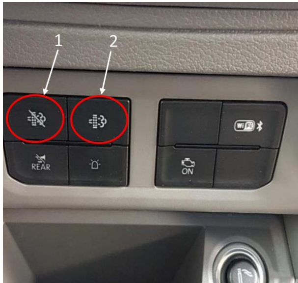
Fig. 1: Parked regeneration button (schematic diagram)
