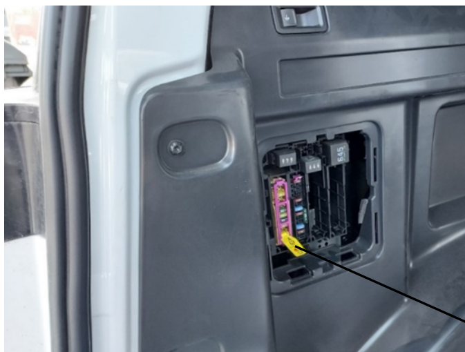
Fig. 1: Position of fuse carrier D in the load compartment on the left behind the trim
