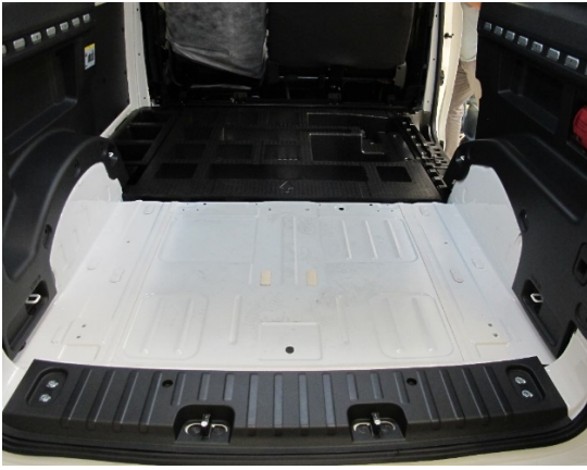
Fig. 3: View of lashing points and bolted connections
