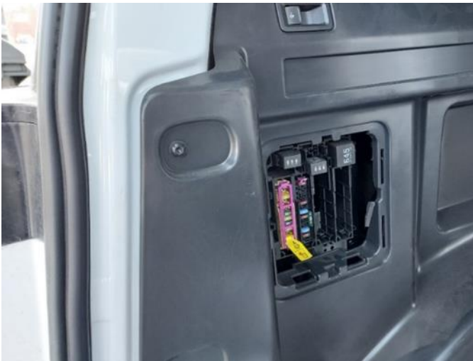
Fig. 1: Position of the fuse carrier in the rear left of the load compartment, behind the trim
