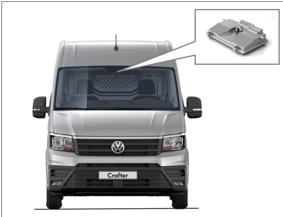
Fig. 1: Position of multifunction camera in vehicle
