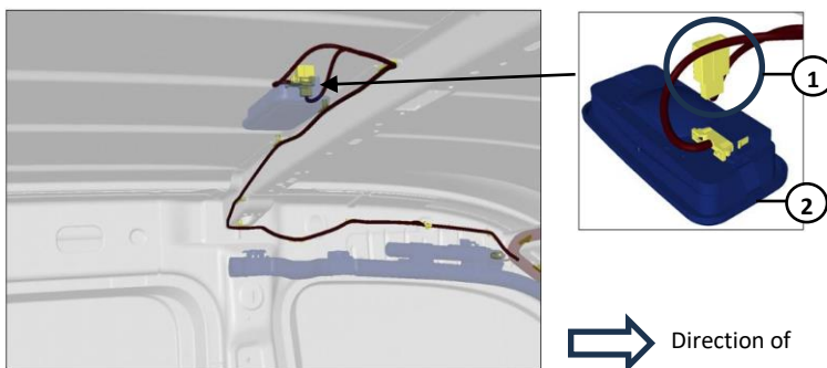
Fig. 4: Position of coupling point for roof, for the rotating light on the double cab
