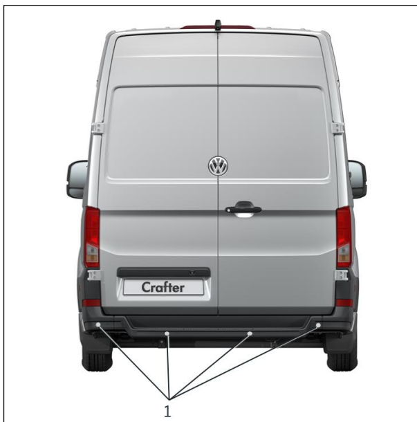
Fig. 2: Position of ultrasound sensors
