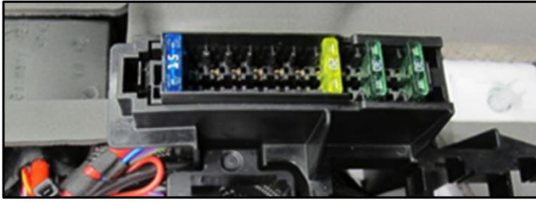
Fig. 3: Detail A: Fuse holder – Connection point for second battery
