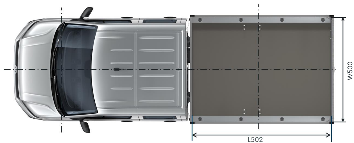
Fig. 2: Vehicle dimensions, single cab, platform van/overhead view
