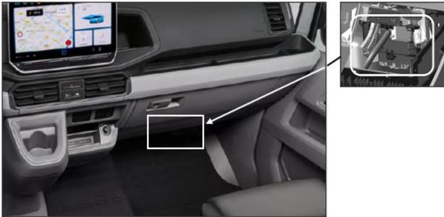
Installation position of the CFCU on the lower dash panel, behind the glove compartment
