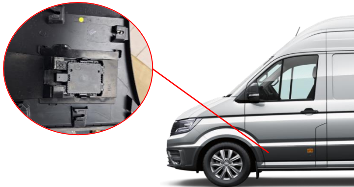
Fig. 3: Position of the radar sensors in the door
