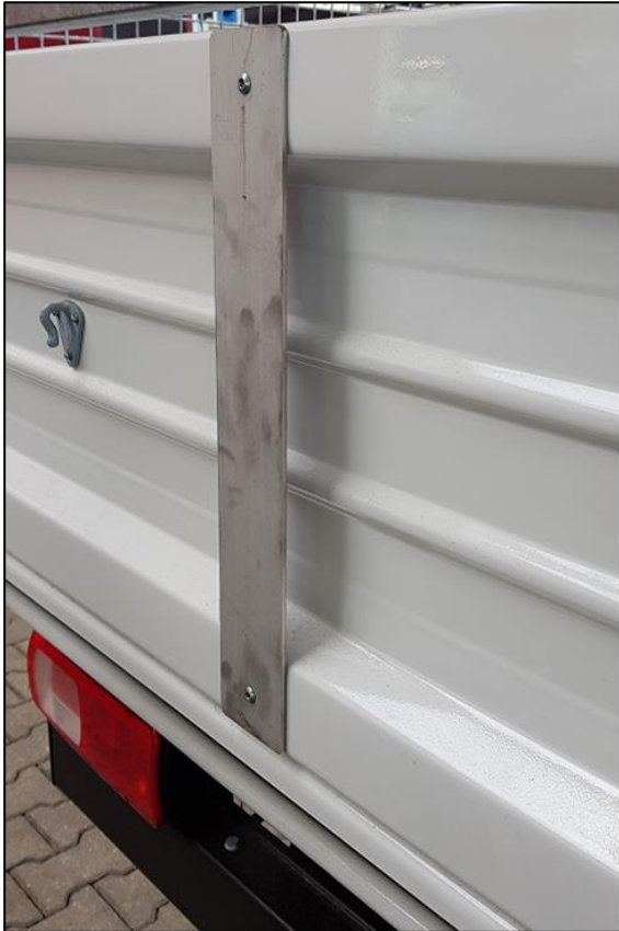
Fig. 3: Wiper plate on rear platform wall
