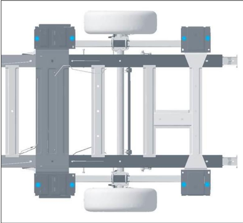
Fig. 7 Crafter flat frame chassis bolting points (schematic diagram of frame area)
