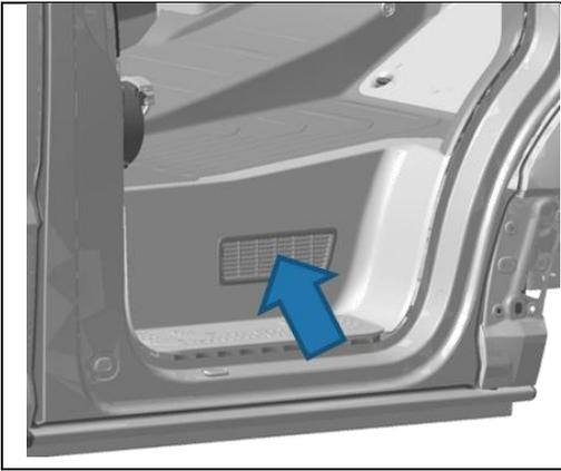
Air intake for auxiliary air heater in the front step to the right
