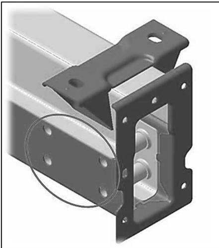
Longitudinal member with holes (diameter: d=14 mm)
