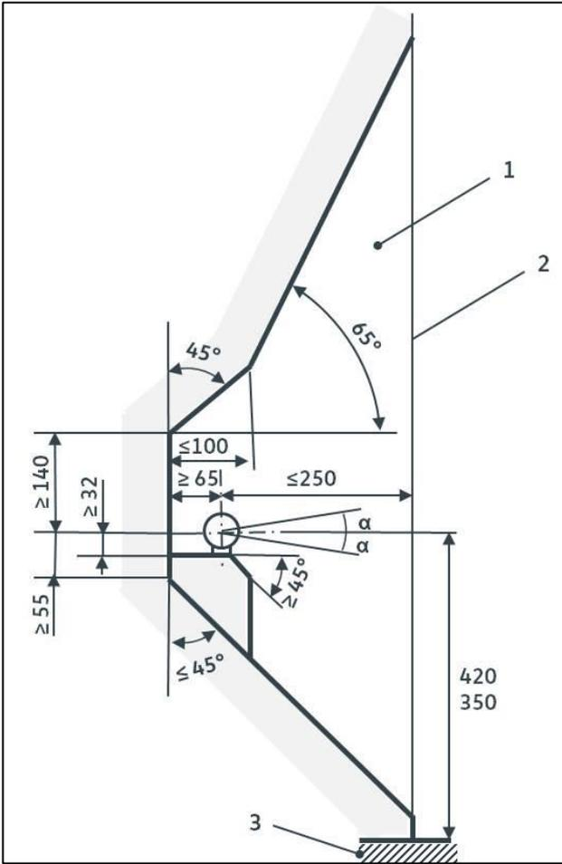
Clearance and height of the coupling ball as per UNECE R 55 (side view)
