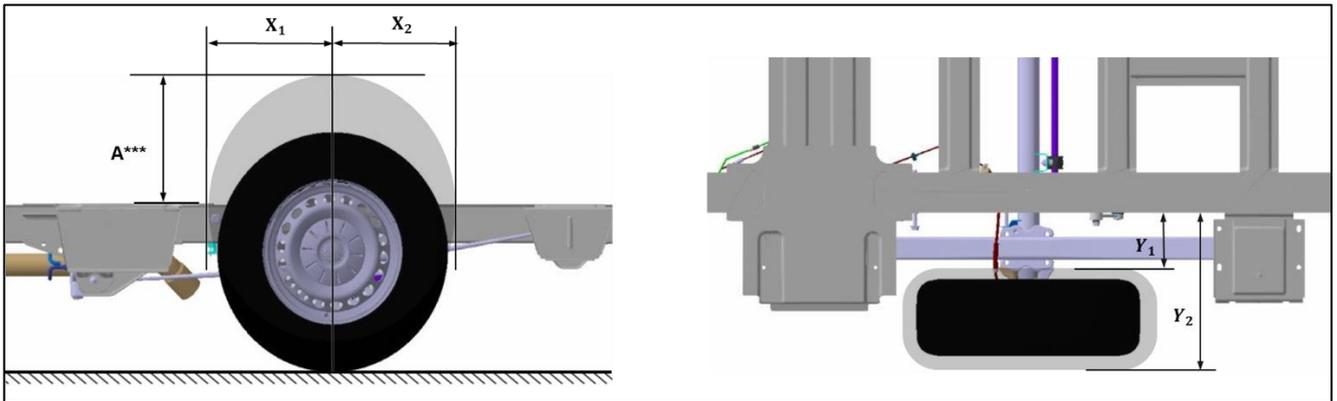
Fig. 1: Limit values for wheel housing clearance requirements
