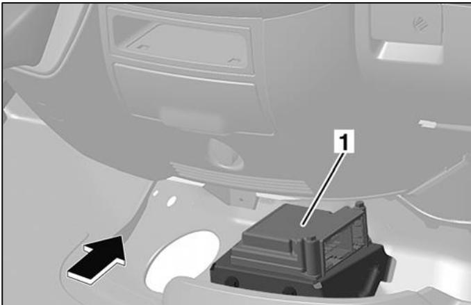
Position of airbag control unit (schematic diagram!)
