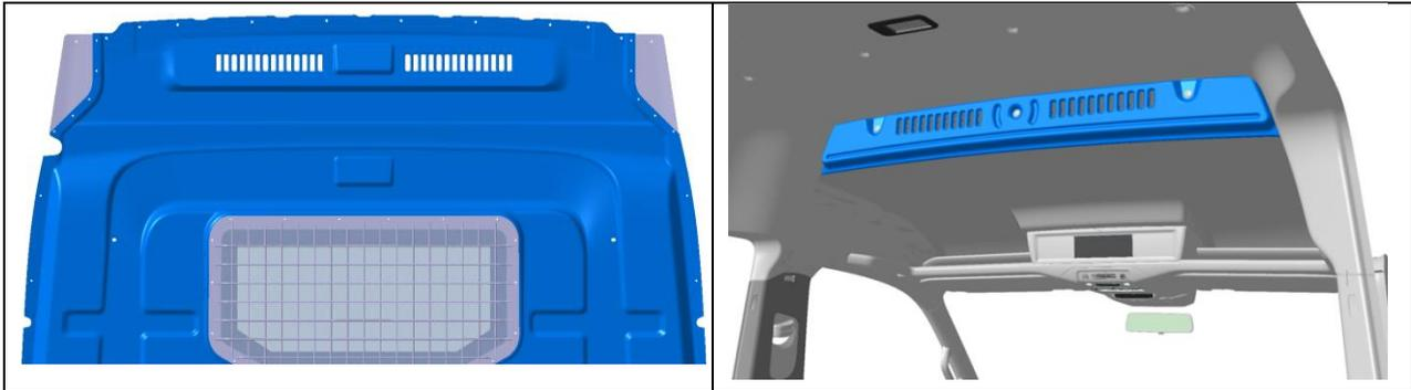
Versions of the air outlet grilles in panel vans with and without a partition
