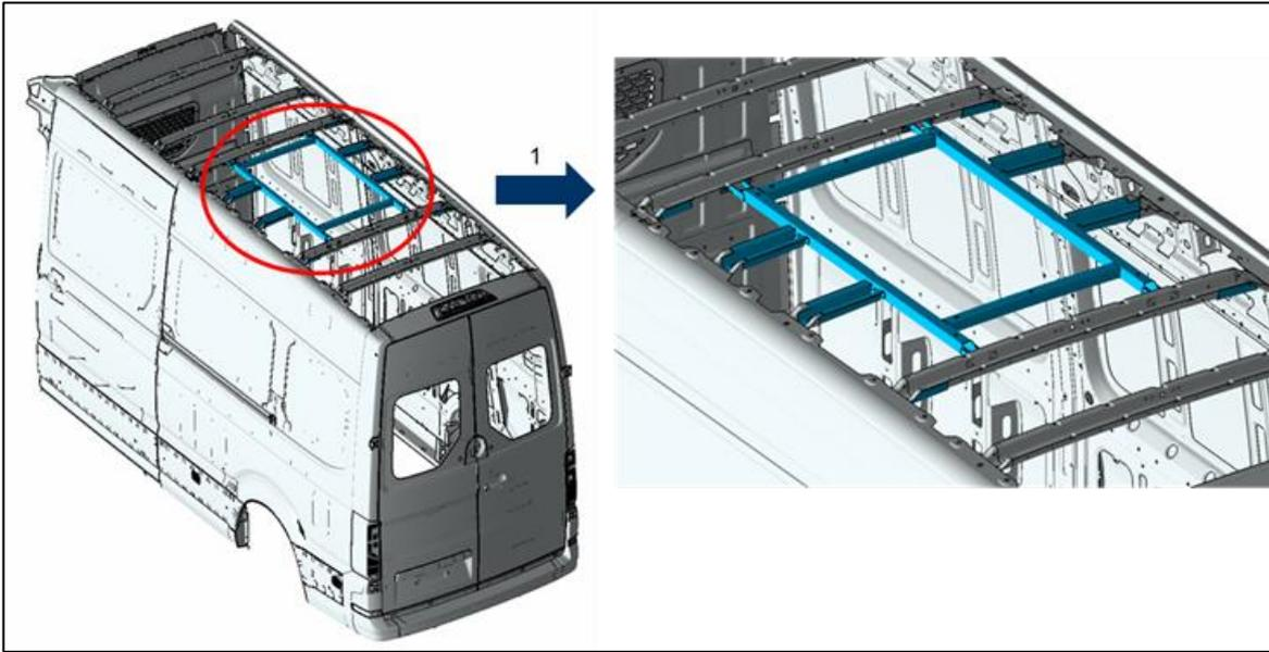
Fig. 2: Preparation for escape hatch (PR no. 3JN)
