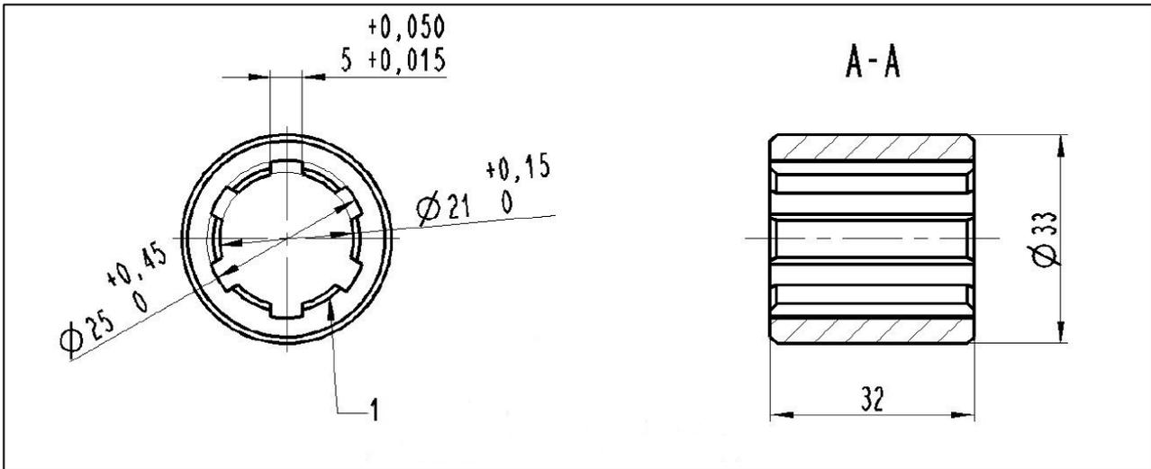
Connection dimensions of splined shaft (1), ISO 14-6x21x25
