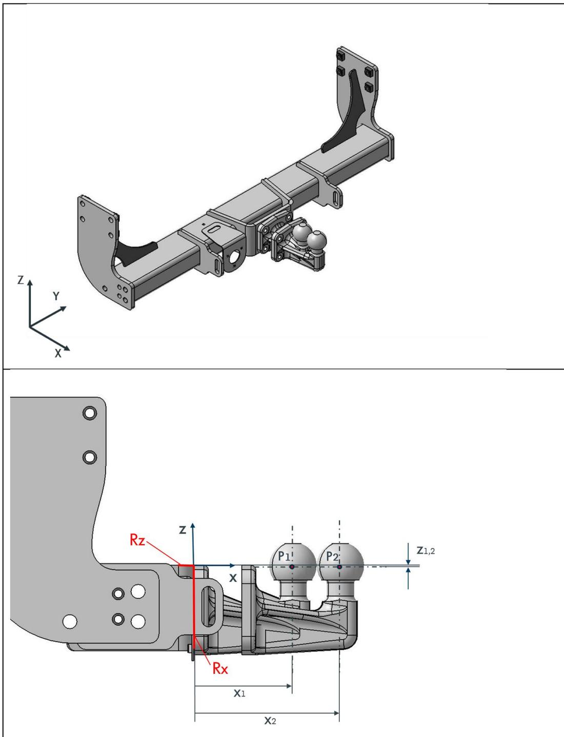
Position ball coupling: rigid towing bracket (P1) and removable towing bracket (P2)
