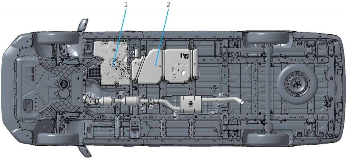
Fig. 1: Installation position of the SCR tank in the vehicle (schematic diagram, vehicle with front-wheel drive)
