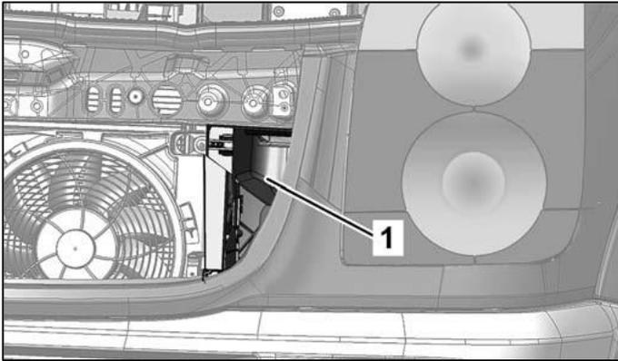
Opening for engine air intake (schematic diagram)
