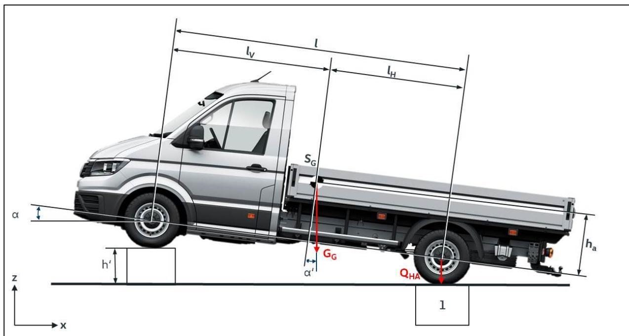
Determining the height of the centre of gravity
