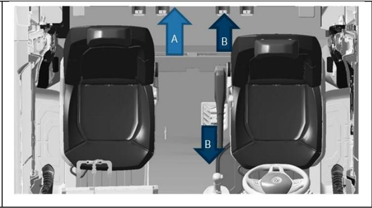
Air outlets for 2nd heat exchanger (A) and auxiliary air heat (B) (panel van without partition)
