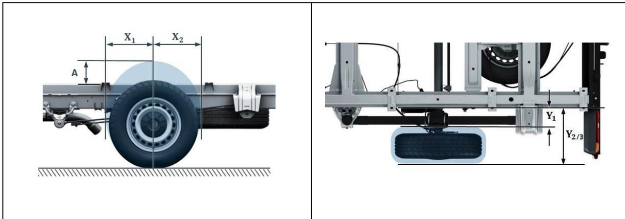
Fig.1 Limit values for wheel housing clearance requirements
