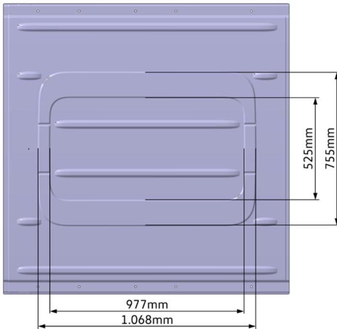
Fig. 3: Dimensions of embossed areas on the high roof
