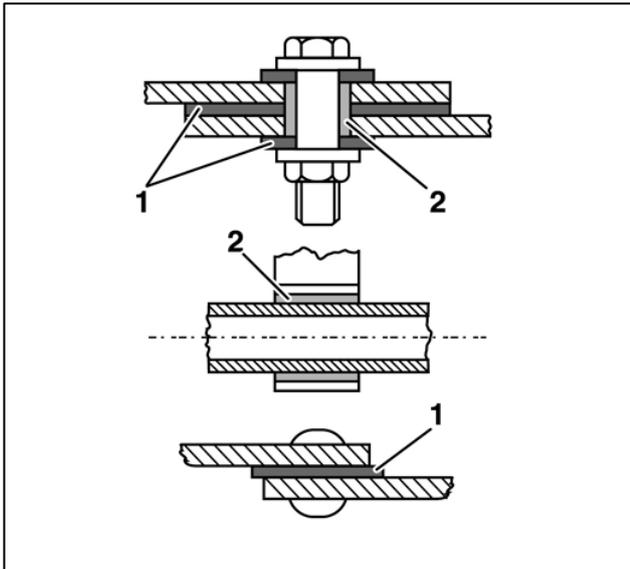
Avoiding contact corrosion
