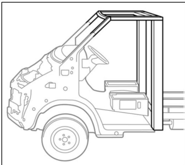
Fig. 10 Example construction of platform with cell structure (schematic diagram)
