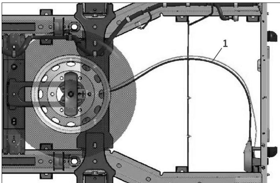
Fig.1: View of spare wheel with bowden cable (1)
