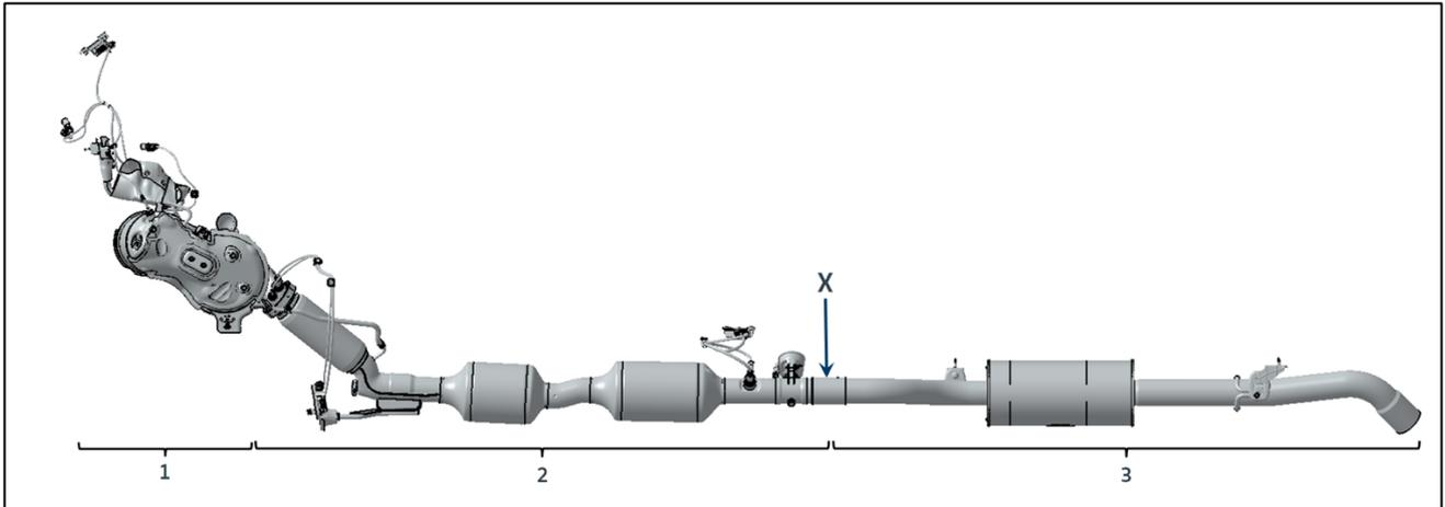
Fig. 3 Emission control section (engine: front-wheel drive/transverse installation), (schematic diagram)
