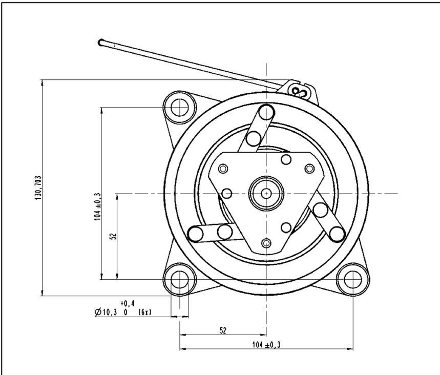
Dimensions of the air conditioner compressor (7C0.816.803), front view
