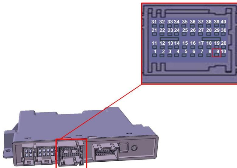
Pin assignment for CFCU connector 3
