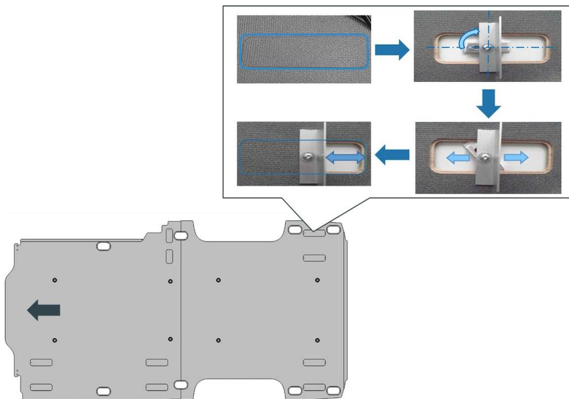
Fig. 2 Universal floor mounting points for storage and shelving system (pictured: wheelbase L3 3,640 mm with sliding door on right)
