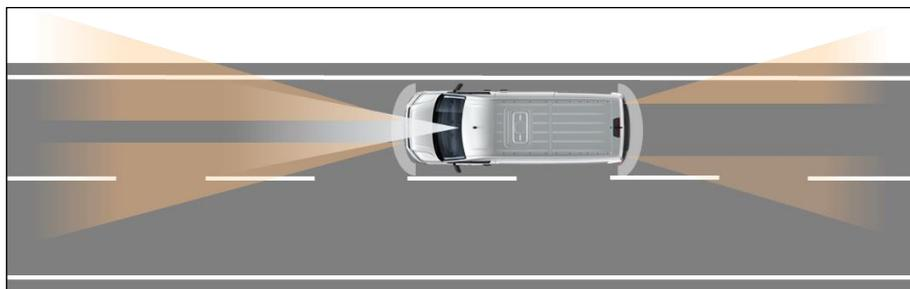
The Crafter features several radar and camera sensors that record the area around the vehicle and analyse it based on intelligent algorithms:
