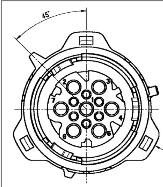
Fig. 1: Coupling point TDSK3 (round connector) - PIN assignment
