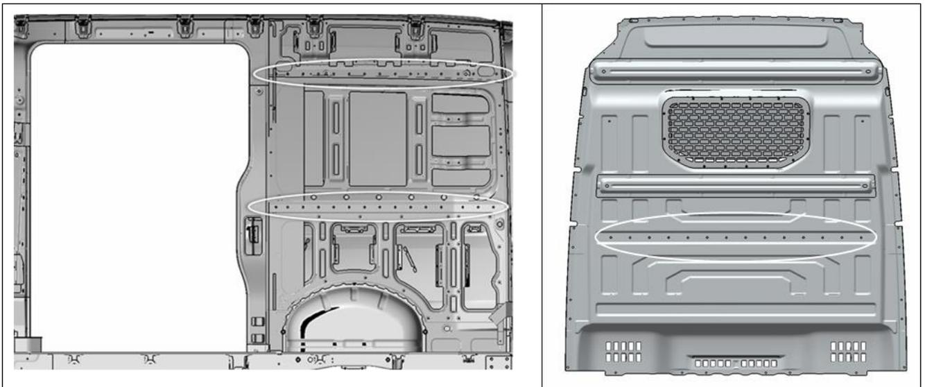
Fig. 3 Preparation for shelving on vehicle body (right sidewall and partition)
