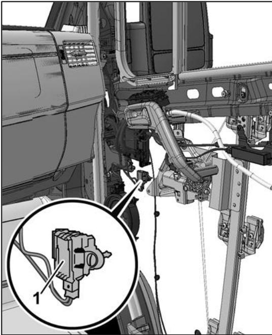
Front pressure sensor (schematic diagram)
