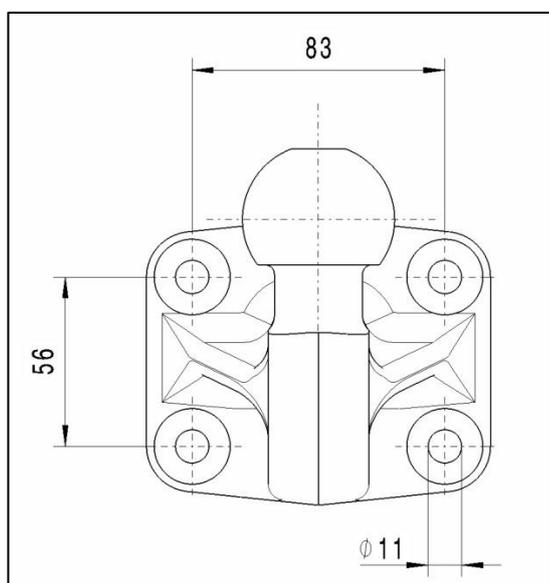
In order to attach the tow hitch, the original hexagonal flange screws, size M10x45-10.9 (N.106.999), must be used.
