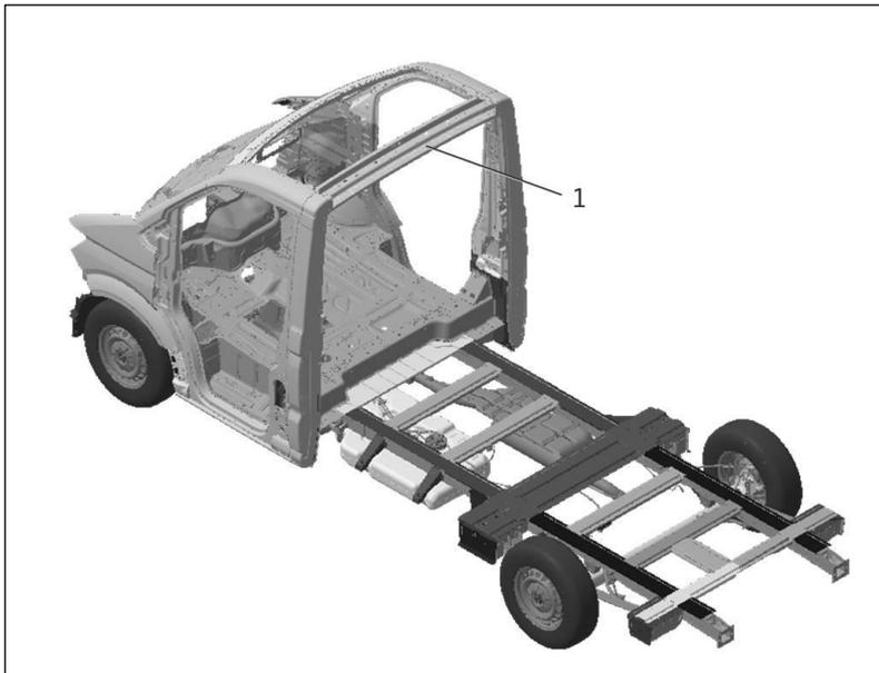
Fig. 2: Cowl panel with flat frame chassis (K4Z)/1-auxiliary roof cross strut for transport
