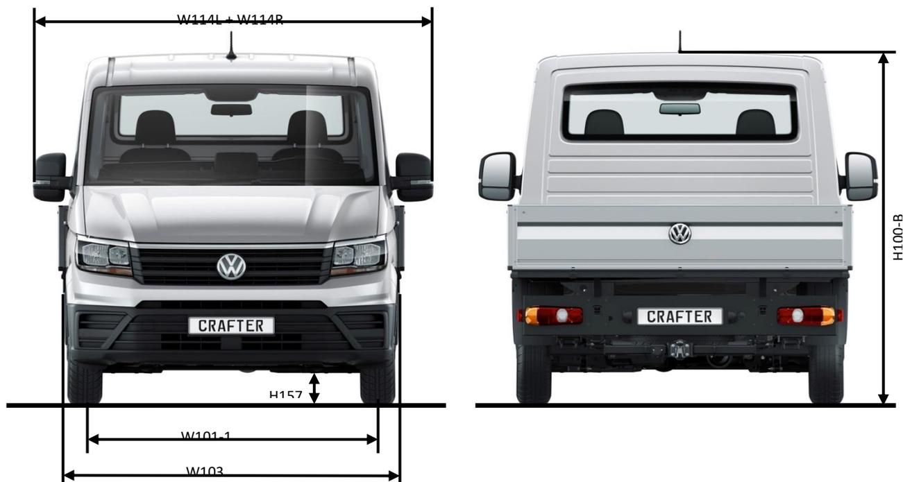
Fig. 3: Vehicle dimensions, single cab, platform van/front and rear view
