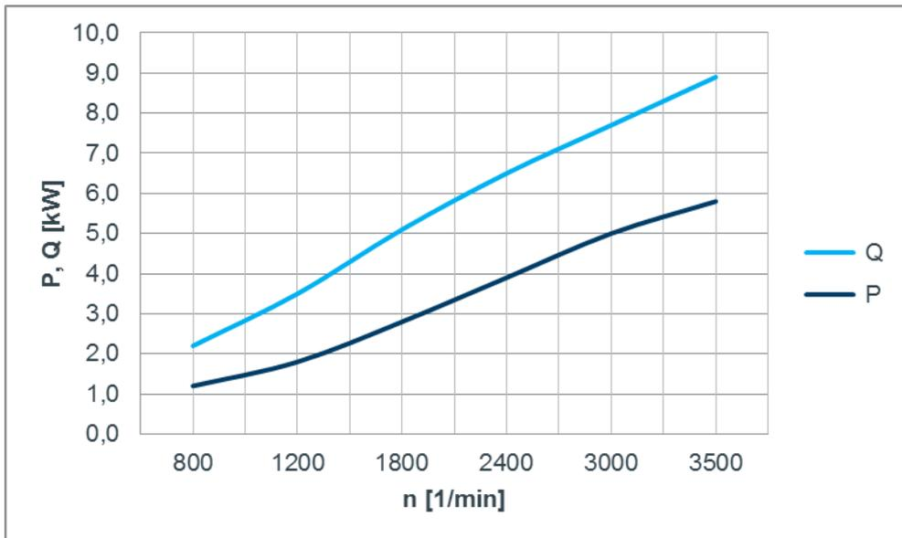
Cooling capacity air conditioner compressor TM16
