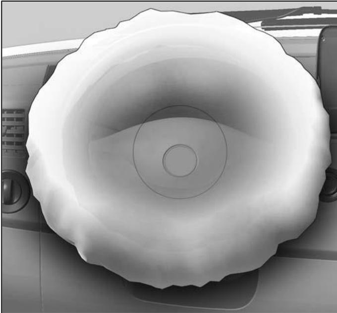
Deployment zone of driver airbag (schematic diagram)
