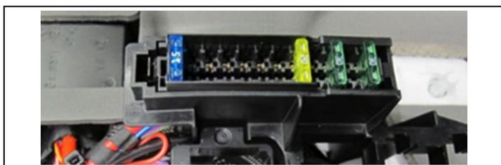
Detail A: Fuse holder – Connection point for second battery
