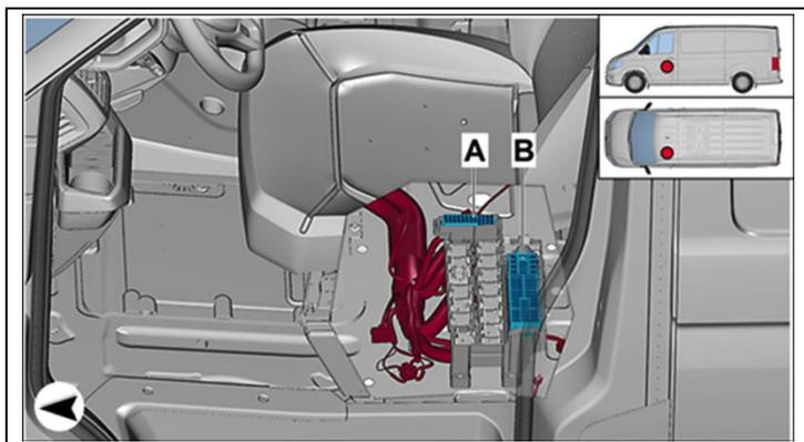
Installation location of fuse holder in the driver's seat (source: Crafter wiring diagram)
