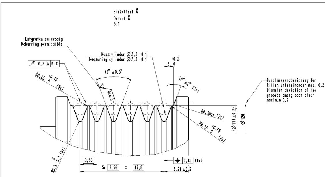
Detail X: Dimensions of pulley for belt 6pk poly-V
