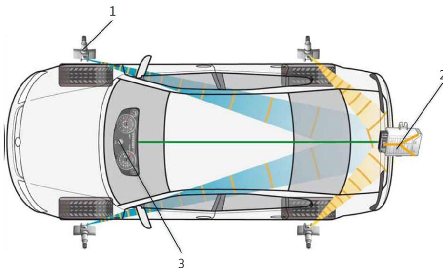
Principle of operation of tyre pressure monitoring system
