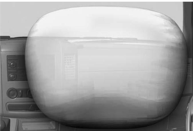
Deployment range of front passenger's airbag (images in progress)
