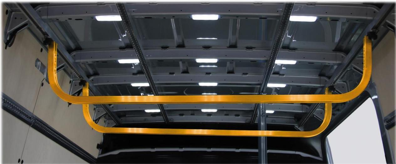
Fig. 1: Vehicle interior roof rack
