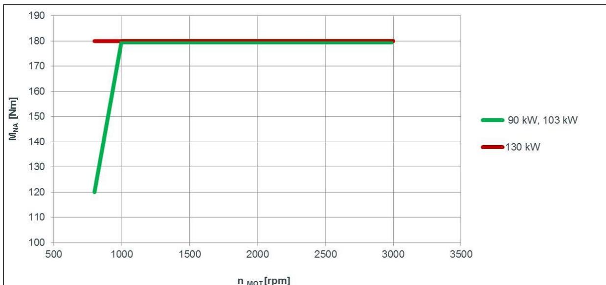
Max. torque  $M_{NA}$  for power take-off dependent on engine speed (engine version 90/103KW and 130KW)
