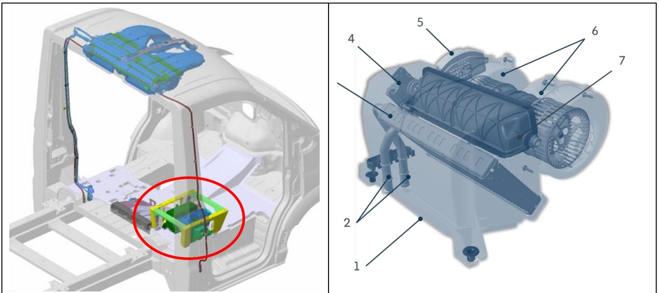
Second heat exchanger with engine coolant connection (heat is drawn from the engine coolant)
