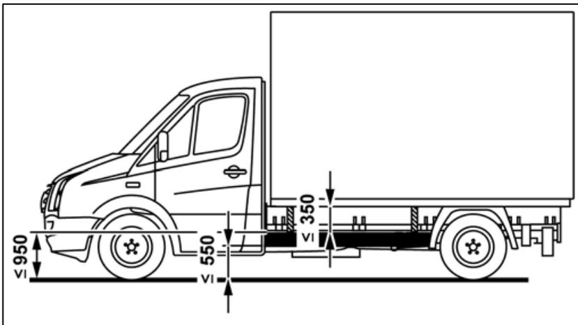
Fig. 1: Position of side guard (schematic diagram)
