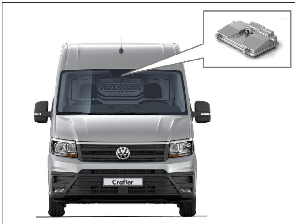
Fig. 1: Position of multifunction camera in vehicle
