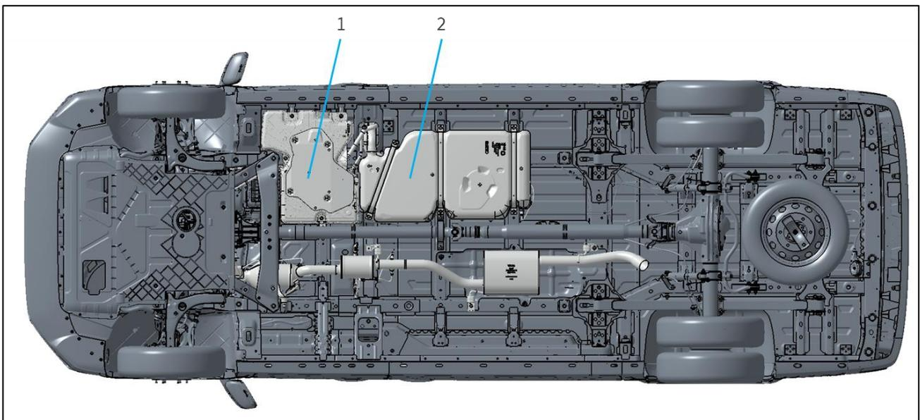
Fig 2: Installation position of the SCR tank in the vehicle (schematic diagram, vehicle with rear-wheel drive), enlarged SCR tank. To be used from the 3rd quarter 2022 for rear-wheel drive.
