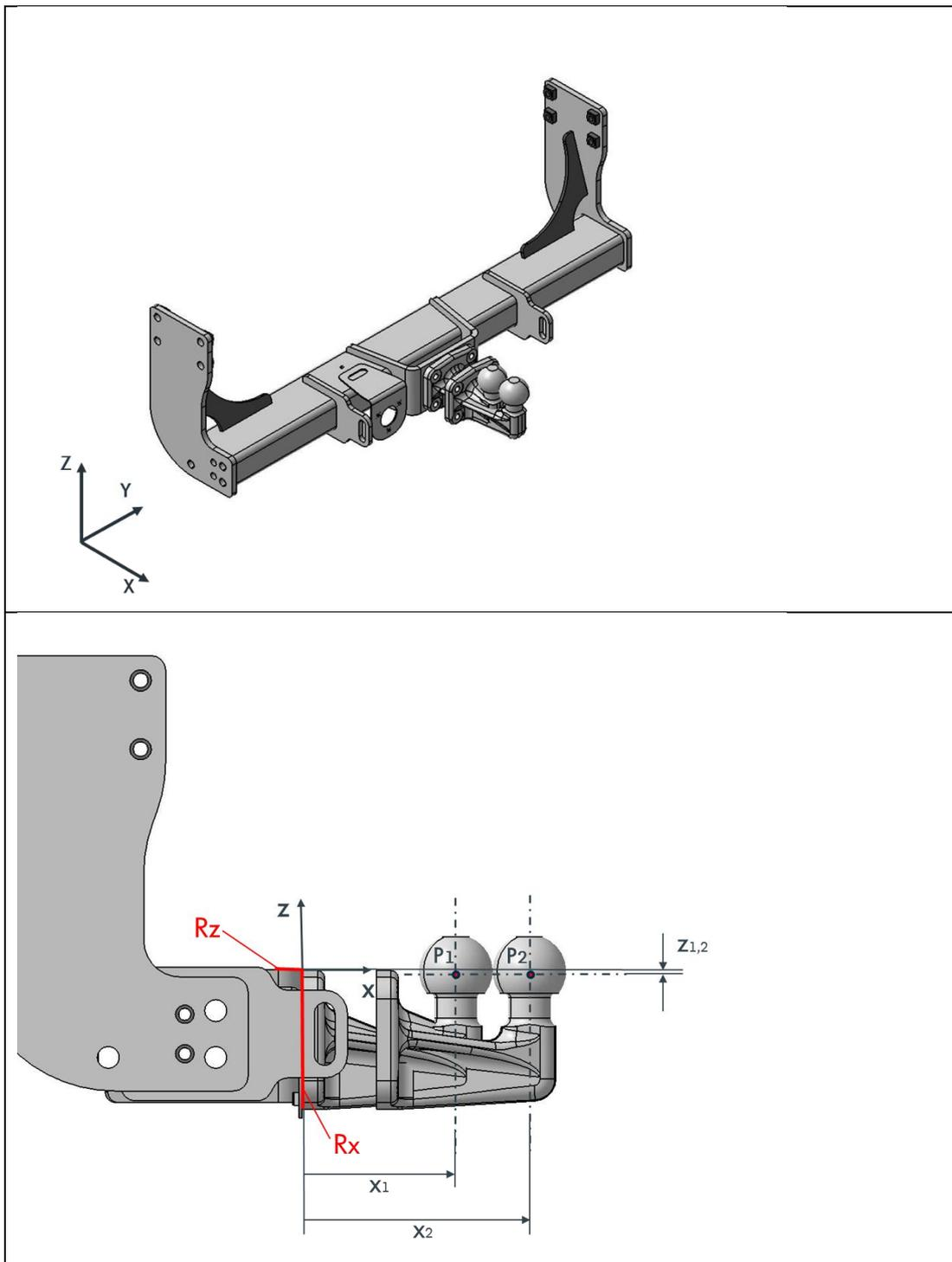
Position ball coupling: rigid towing bracket (P1) and removable towing bracket (P2)
