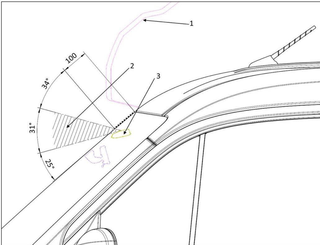
Fig. 2: Limit for add-ons to vehicles with a front camera
