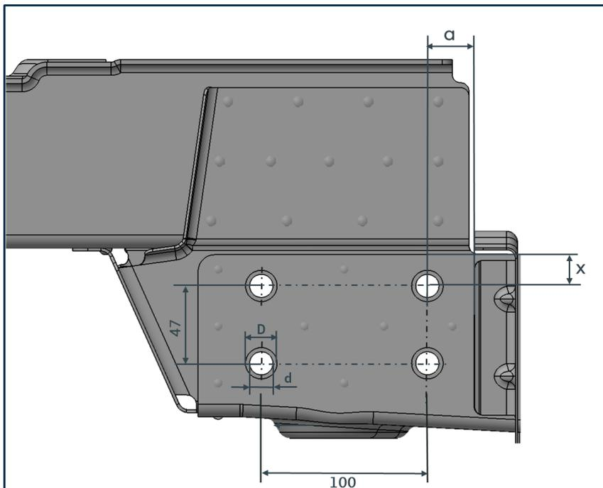
Fig. 2: Panel van/window van, 3.0 – 5.50 t (high floor)
