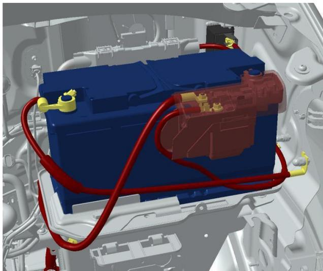
Second battery installation position, on left in engine compartment when viewed in direction of travel
