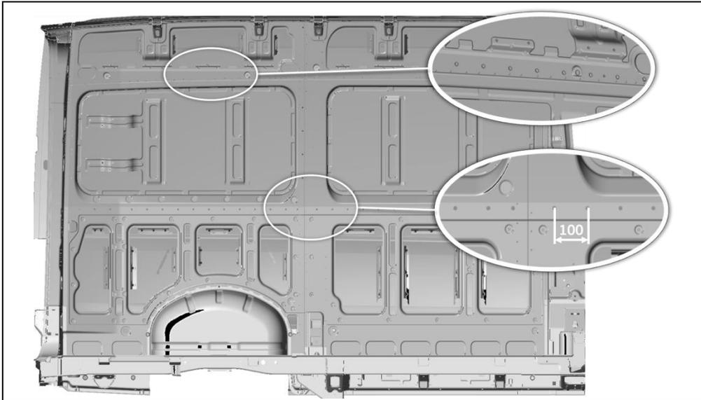
Fig. 2 Preparation for shelving on vehicle body (left sidewall), hexagonal bore hole spacing 100 mm
