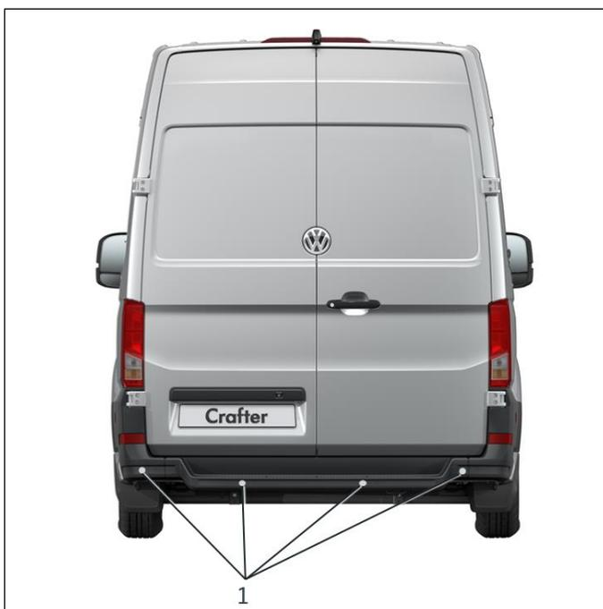
Fig. 1: Position of ultrasound sensors
