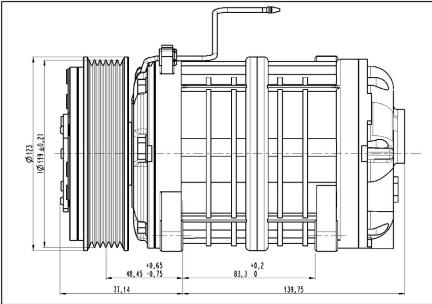
Dimensions of the air conditioner compressor (7C0.816.803), side view
