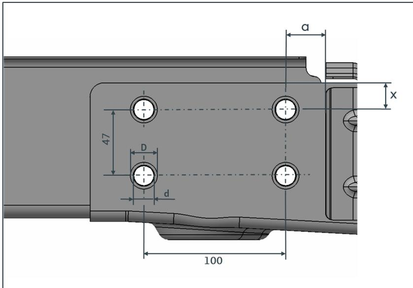
Fig. 1: Panel van/window van, 3.0 – 4.0 t (low floor)
