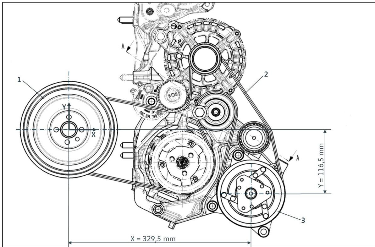
Drive formation additional air conditioner compressor, dimension between axes to crankshaft pulley
