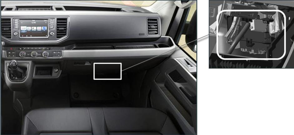
CFCU installation position on the right of the dash panel
