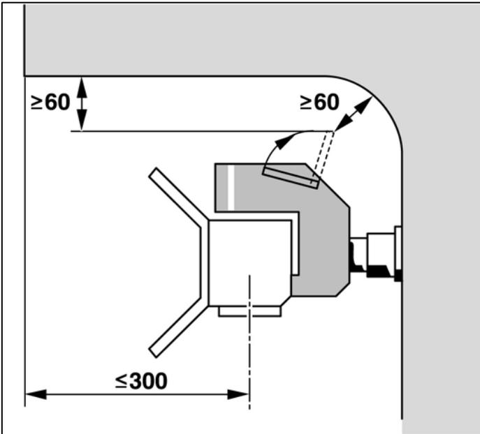
Hand lever clearance for pin coupling as per UNECE R 55 (side view)
