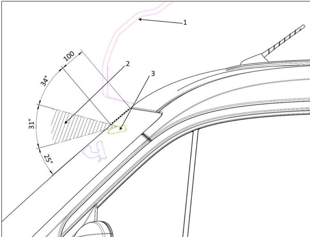
Fig. 1: Limit for add-ons to vehicles with a front camera
