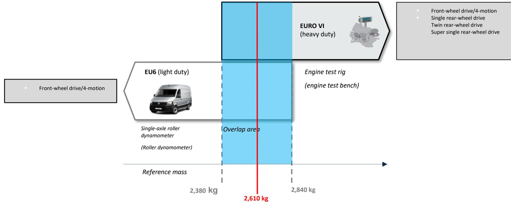
Light duty: Single-axle roller dynamometer test: can be used up to max. <RM 2,610 kg
