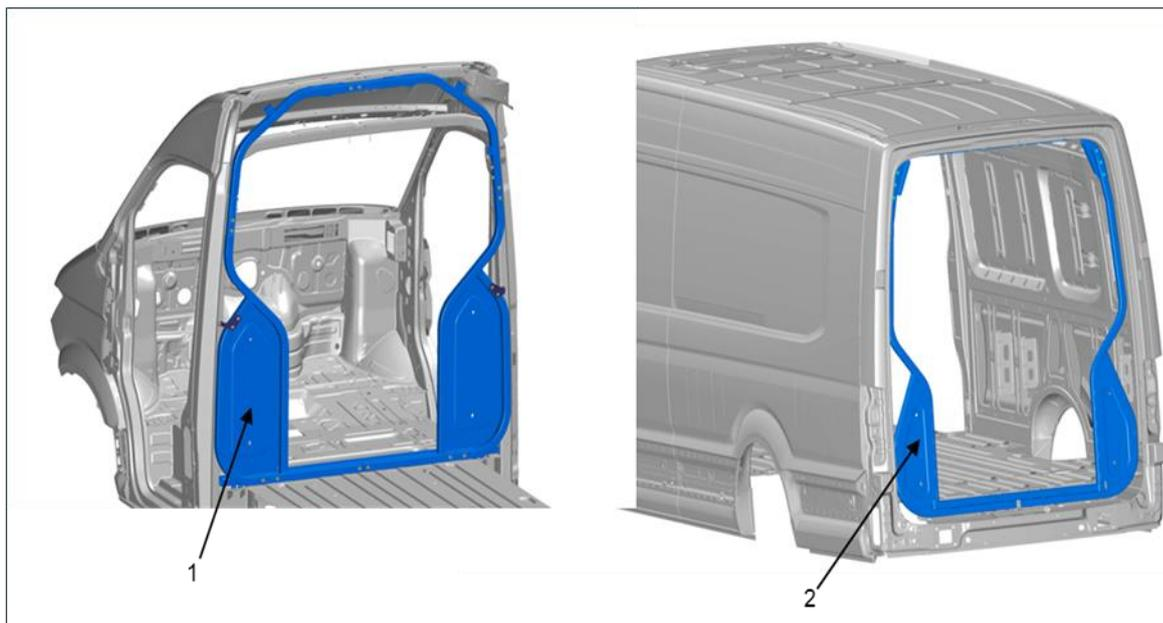
Fig. 1: Roll bar (PR no. 2Y1)
