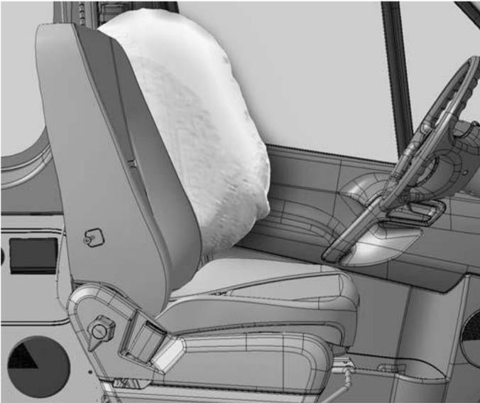
Deployment zone of thorax bag on left of vehicle (schematic diagram)
