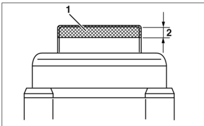
Fig. 2: Painting area of cylindrical sensor membrane edge
