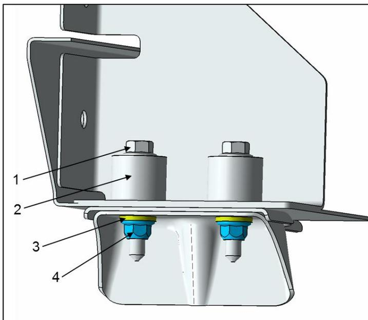
Fig. 2 Construction example: bolted connection with damping element
