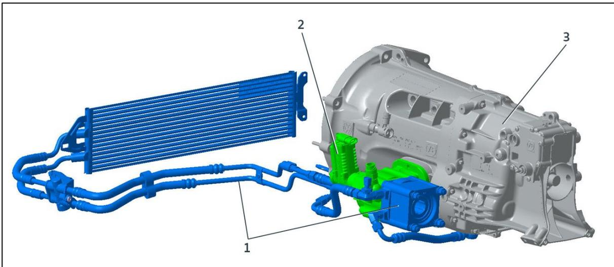
Fig. 1 Power take-off system with gear oil cooler (PR number: OR4)
