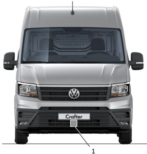
Fig. 1: Radar delantero
