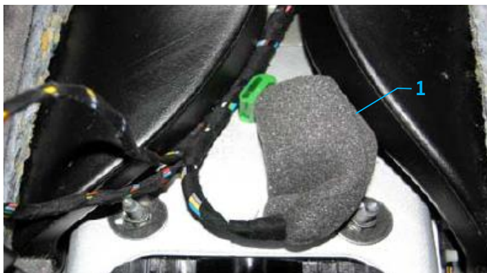
Fig. 3: Electrical interface for special vehicles, View R (PR number IS1/UE1 cable 2K5.970.372)
