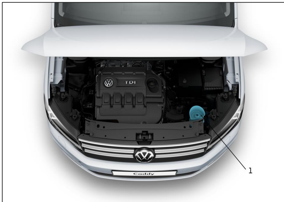
Fig. 2 Filling opening of the AdBlue® tank in the engine compartment
