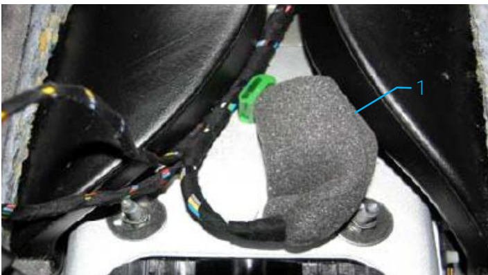
Fig. 3: Electrical interface for special vehicles, View R (PR no. IS1/UE1 cable 2K5.970.372)
