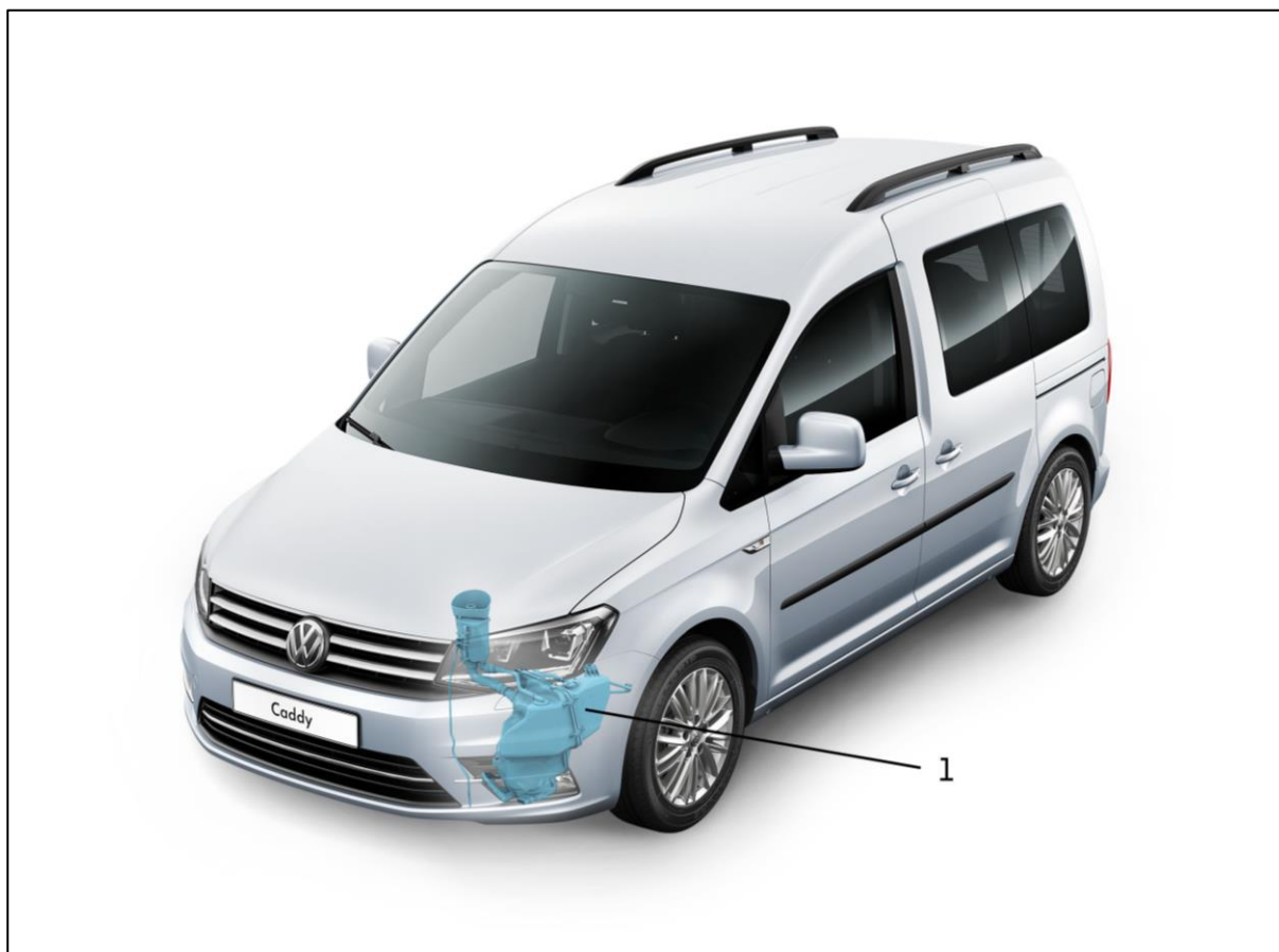
Fig.1 Installation position of the AdBlue® tank in the vehicle
