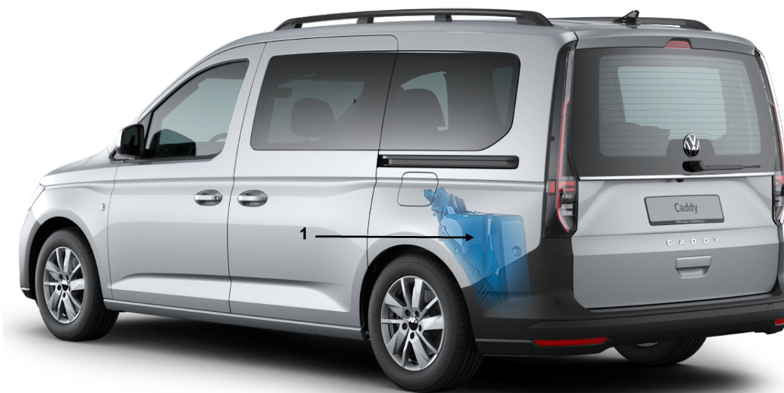
Fig. 1 Installation position of the reducing agent tank in the vehicle
